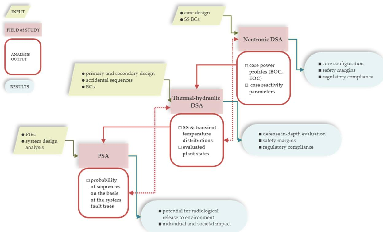
**Figure 3.** Flow diagram of the GOSPOSTRATEG-HTR safety analysis methodology in the Phase B Stage 5. DSA – Deterministic Safety Analysis. PSA – Probabilistic Safety Analysis.
