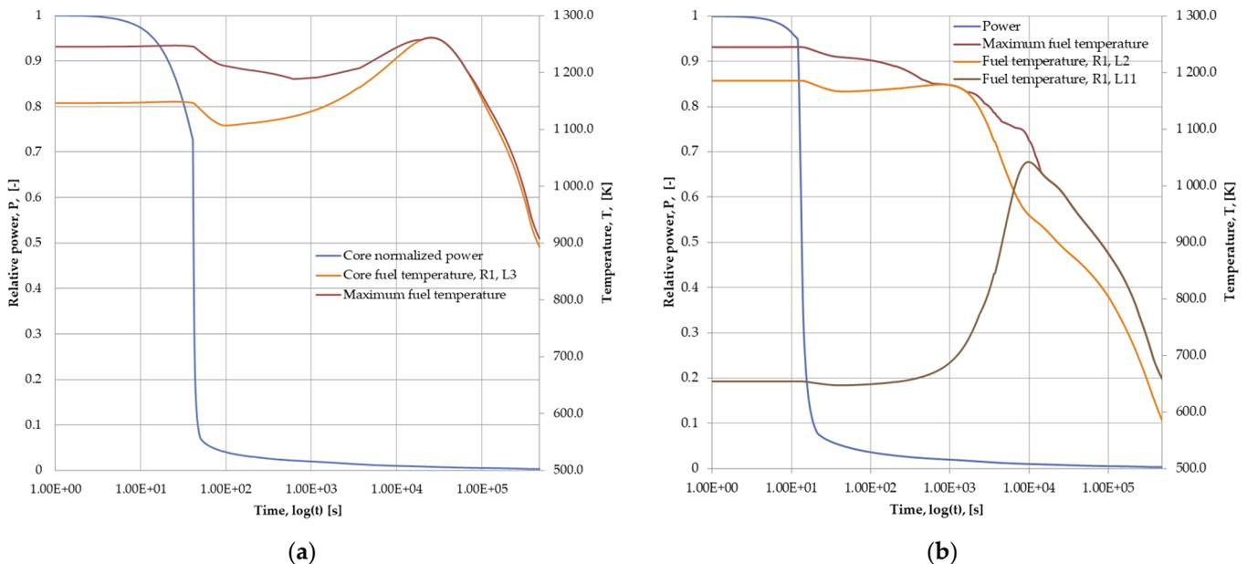
**Figure 6.** DLOFC (a) and PLOFC (b) accident core normalized power ( $P$ , [-]) and fuel maximum temperatures ( $T_f$ , [K]).
