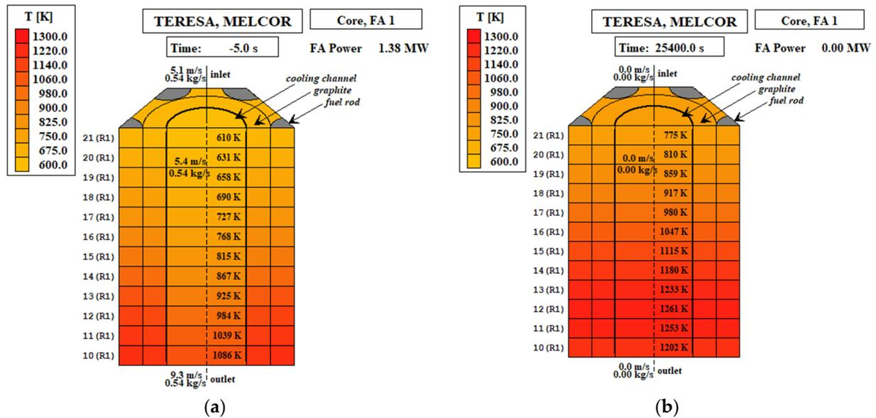
Figure 7. Temperature in the cooling channel of central block of the core: (a) steady state (5 s before accident initialization); (b) DLOFC conditions,  $T_{max}$  at  $t = 25,400$  s (BOL case).
