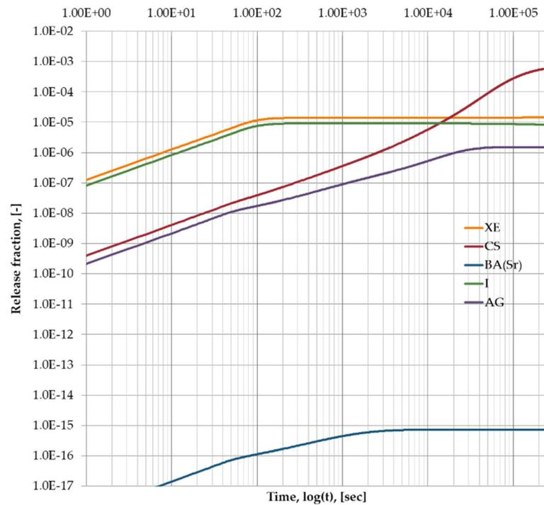
**Figure 5.** TRISO fuel release fraction of the core inventory for selected radionuclide groups. MELCOR2.2 results for DLOFC accident with inventory at EOC core state.
