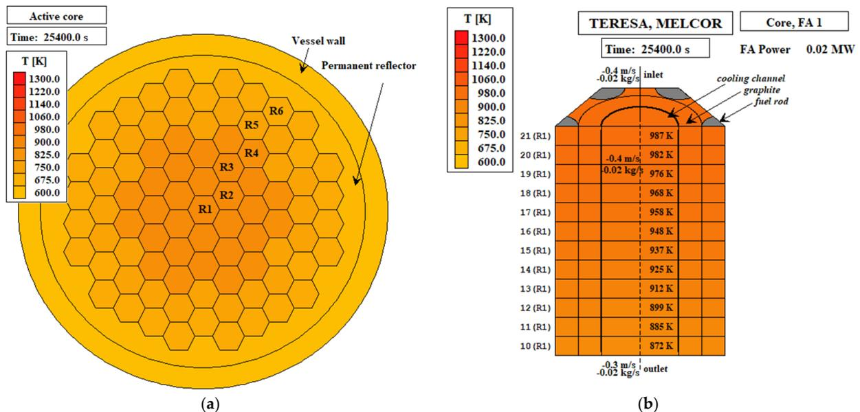
Figure 8. Results of PLOFC scenario, at  $t = 25,400$  s: (a) temperature of the fuel at the bottom of the core; (b) temperature of cooling channels in the central block (BOL case).
