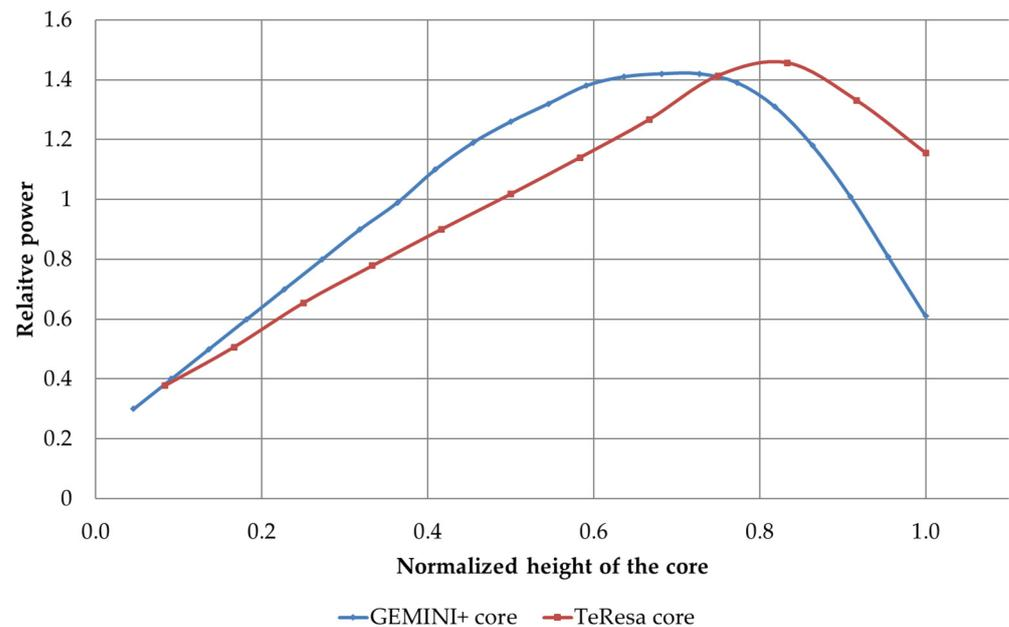
**Figure 4.** The comparison of the axial power distribution for GEMINI+ and TeResa core.
